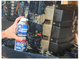
Fog the carburetor/air breather intake(s) with an engine fogging oil. Fogging oil is an anticorrosive mixture that protects the internal surfaces of the carburetor and the cylinders. Available in bulk or aerosol cans, fogging oil is formulated to stick to the cylinders and not slide down the walls. Follow the instructions that come with the product. Remove the cowls of your motor, and spray the fogging oil into the intake holes/vents.
