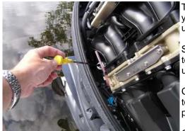
Touch up damaged paint (you can usually get a perfect color match paint from your dealer or from an automotive paint store. Mist-coat powerhead and any unpainted parts with an anticorrosion spray.
