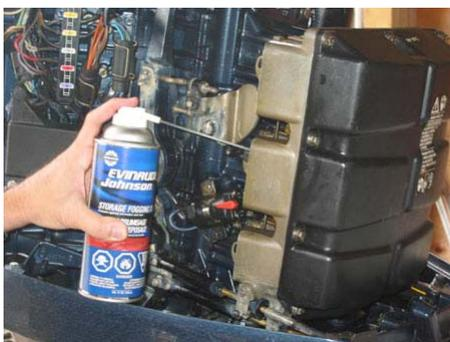
Fog the carburetor/air breather intake(s) with an engine fogging oil. Fogging oil is an anticorrosive mixture that protects the internal surfaces of the carburetor and the cylinders. Available in bulk or aerosol cans, fogging oil is formulated to stick to the cylinders and not slide down the walls. Follow the instructions that come with the product. Remove the cowls of your motor, and spray the fogging oil into the intake holes/vents.
