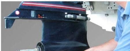
Even a small leak in your bearings or shaft seals will allow moisture to migrate into your gearcase. The carbon-steel parts, like gears and some shafts, will corrode, and ultimately cause more seal failures. But worse - if there is any water or moisture whatsoever inside your gearcase, the result can be a cracked housing! It is easy
