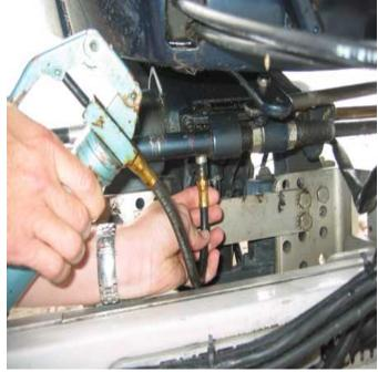
mechanisms. Pumping some grease into these areas will displace any water that might be there.
